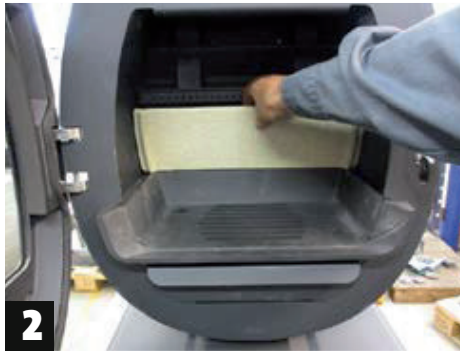
2 Slide the plate behind the grate
